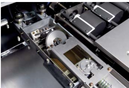
Automated Point Spine Glue: Glue Length (Top-Bottom), Wiper Opening for Glue Amount (First Application Roller/Second Application Roller), Spine Glue Thickness (Second Application Roller Height), Side Glue: Side Gluing Roller Width
